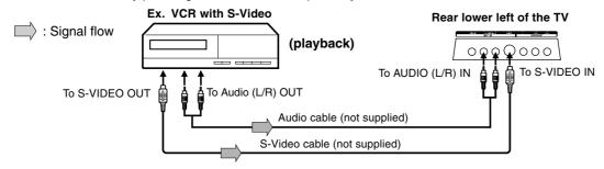
Note: When the S-VIDEO cable and the standard video cable are connected at the same time, the S-video cable takes precedence.
